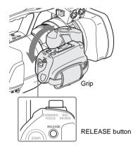
Click positions are provided at each 15 degrees. Release the RELEASE button at the desired click position to lock the grip.
